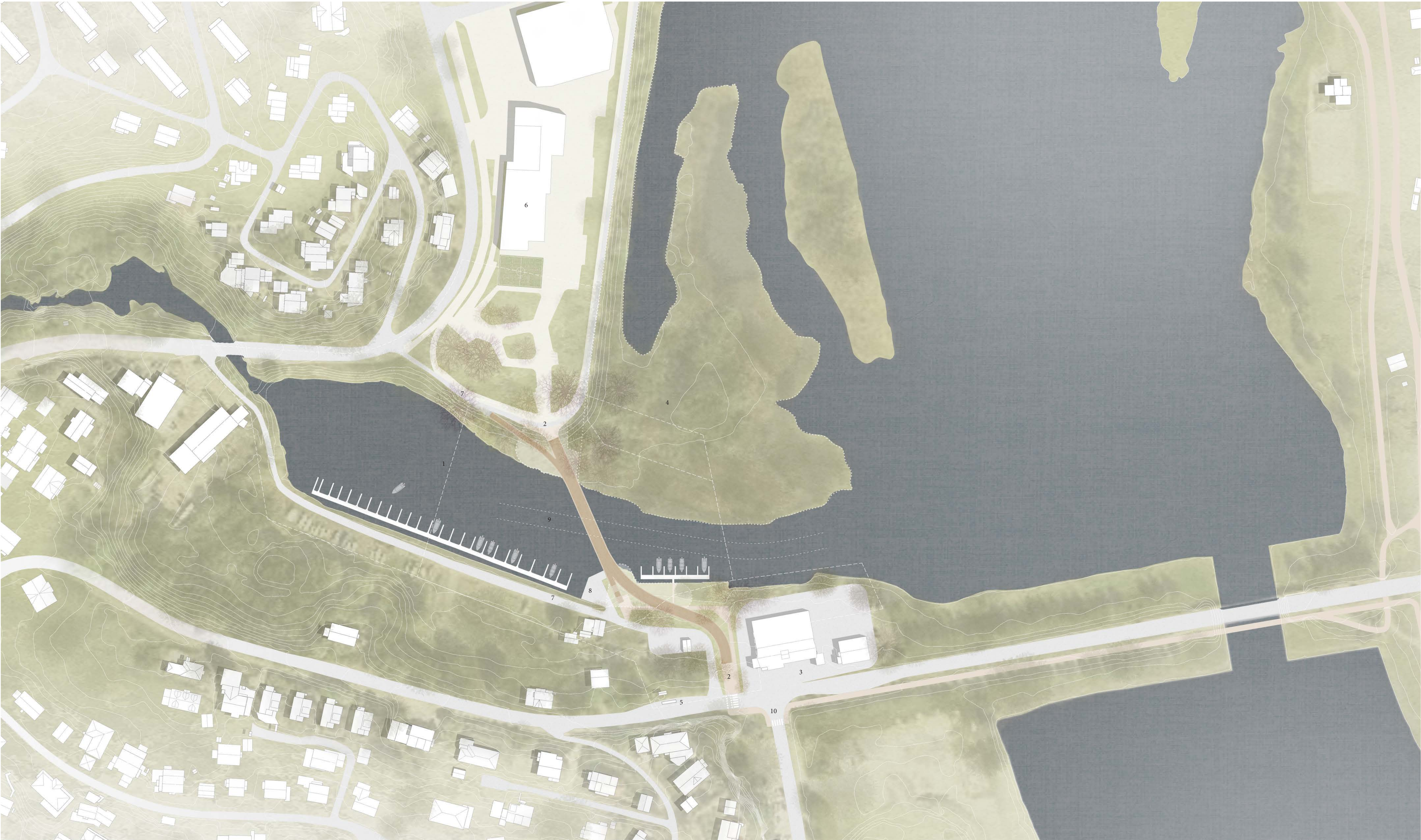
Siteplan 1.Project area 2.Access area 3.Future demolition area 4.Protected area 5.Bus stop 6.School 7.Hiking path 8.Crane truck's space 9.B012 drain line 10.Pedestrian and cycle connection path
