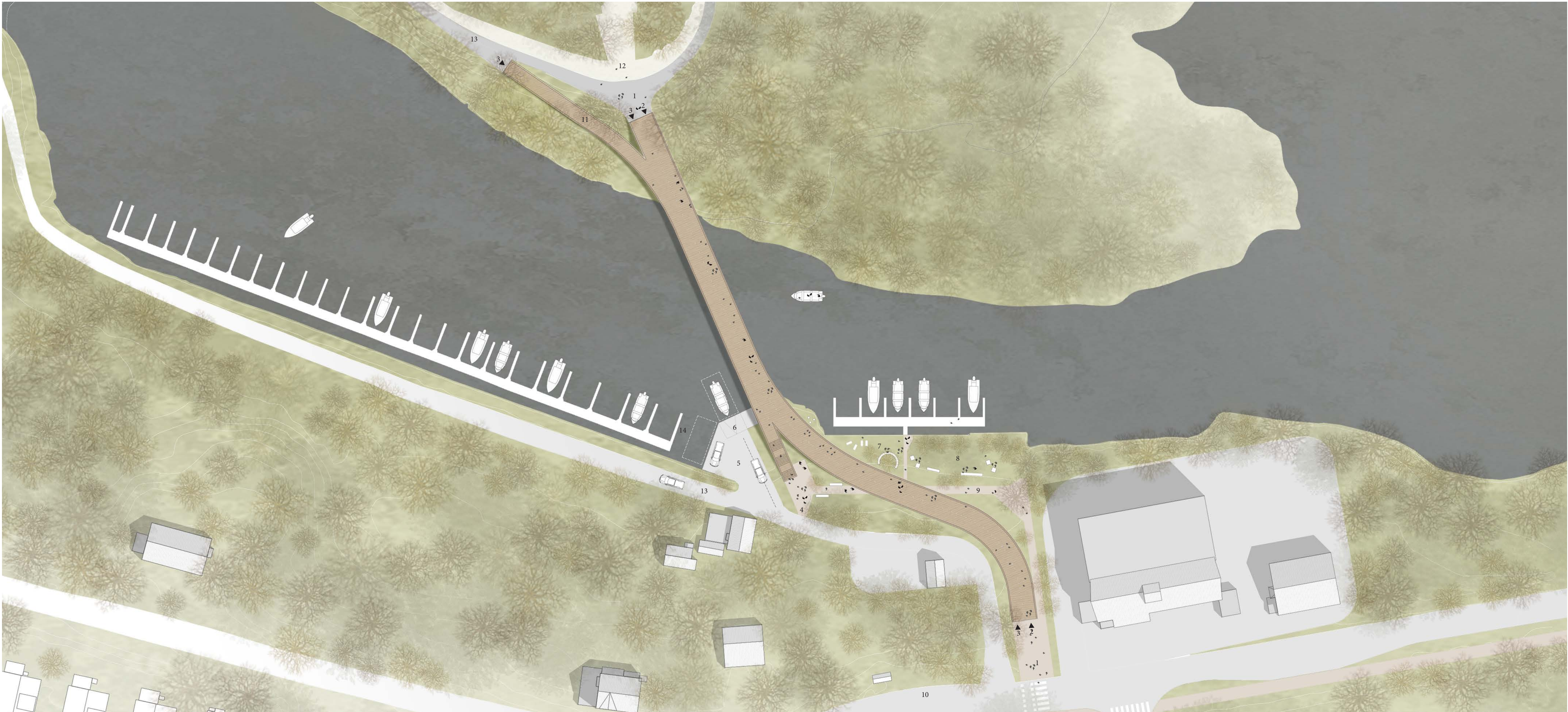
Siteplan 1.Access area 2.Pedestrian access 3.Bike access 4.Connection to the hiking path 5.Crane truck's space 6.Slope 7.Solarium 8.Relax area 9.Pedestrian path 10.Bus stop 11.Bicycle walkway 12.School Entrance 13.Touristic route 14.Repositioning of 2 boat berths
